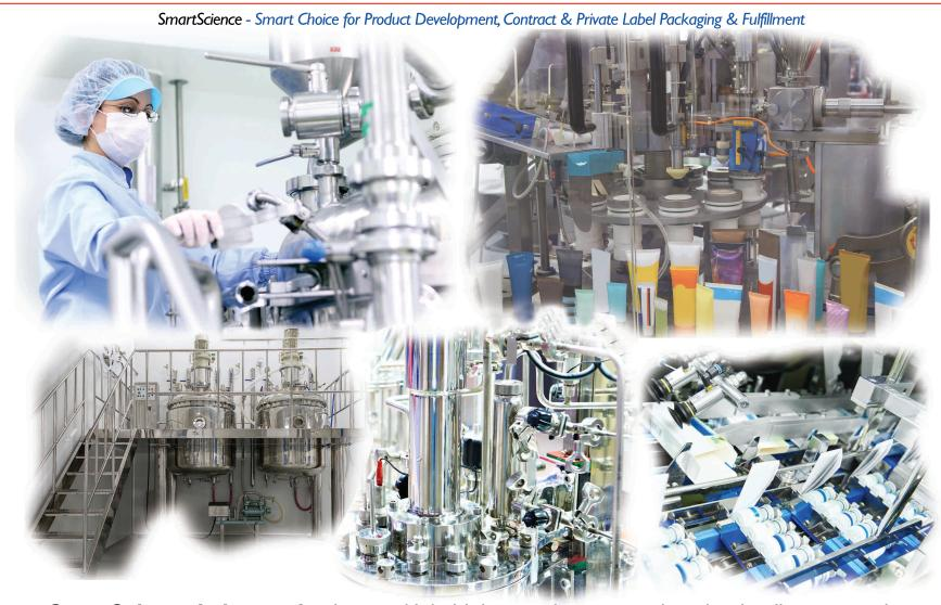
SmartScience Laboratories has multiple high speed automated packaging lines operating at the same time. Plastic tubes and bottles are filled in a variety of sizes and placed into glued or tucked flap retail cartons, shrink wrapped into desired inner-packs, placed into shippers and palletized. SmartScience Laboratories also has high speed automated blister packaging line for packaging of capsules or tablets and much more.
